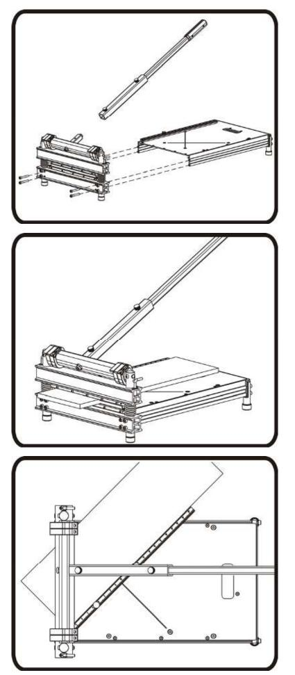
**Installation** Install the table to the cutter base with provided screws and bolts as shown. Then insert the handle into the handle base as show and tighten provided screw.
